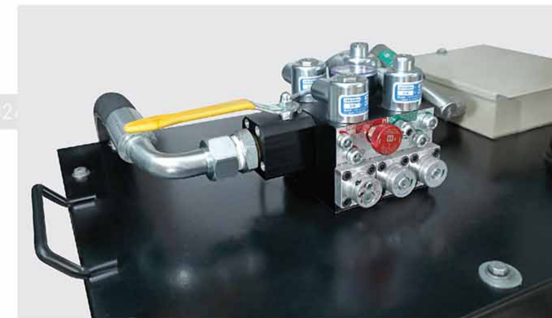
Hydraulic Valve is a solenoid operated check valve designed for hydraulic elevators and includes a self-closing manual lowering valve. Its purpose is to allow free flow of oil from the pump unit to the cylinder for upward travel and to prevent flow in the reverse direction from the cylinder to pump until an electrical signal is given to its solenoid.
